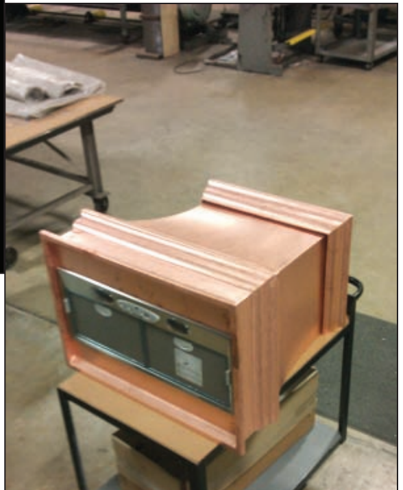
copper hood prior to finishing
